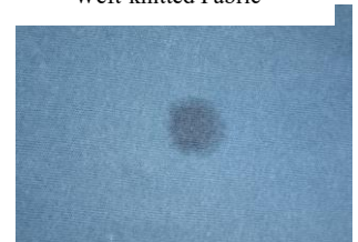
Fig. 4 Oil Stains Defect of Weft-knitted
