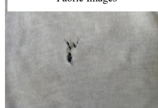
Fig. 3 . Holes Defect of Weft-knitted Fabric
