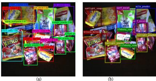
Figure 6 Sample test results for detection of grocery items with overlapping and obscured boundaries where a) shows the detections of YOLOv3 model and b) shows detections of Faster R-CNN model.
